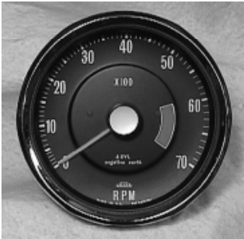
Figure 1: The 7K Alpine tachometer.
